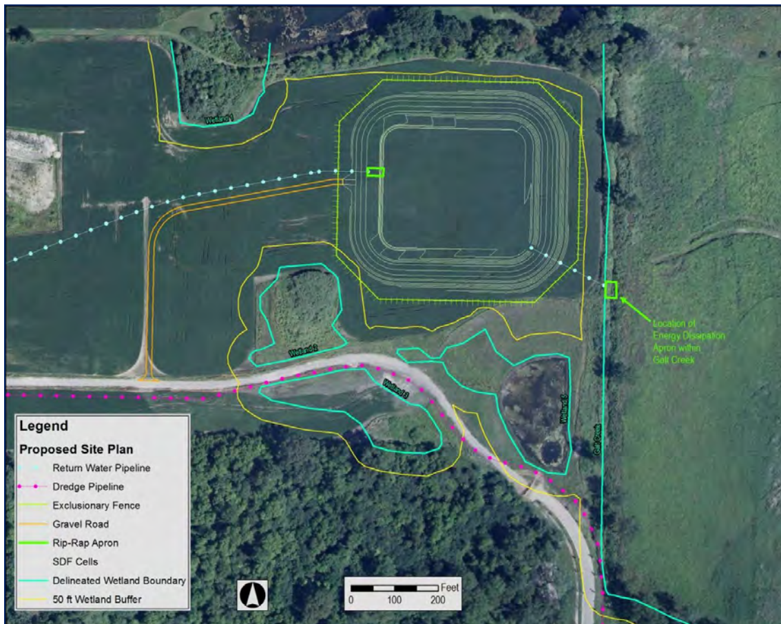
Figure 1: Location of Energy Dissipation Apron
